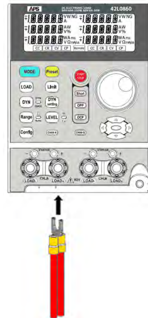
Figure 7-1: Doubling wire size using spade lugs
