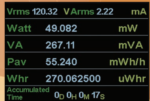
Standby Power Result Display
