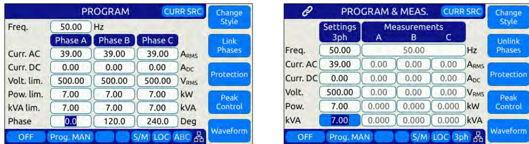
Figure 6-3: PROGRAM Screens Current Source Mode
