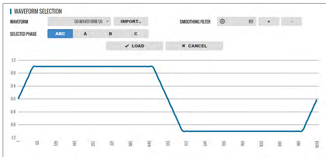
Figure 6-9: Same Waveform with maximum smoothing Filter Applied
