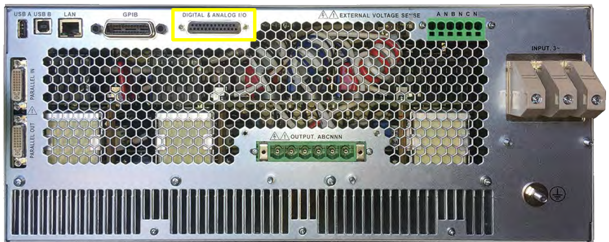
Figure 7-1: Rear Panel AUX I/O DB25 Connector Location
