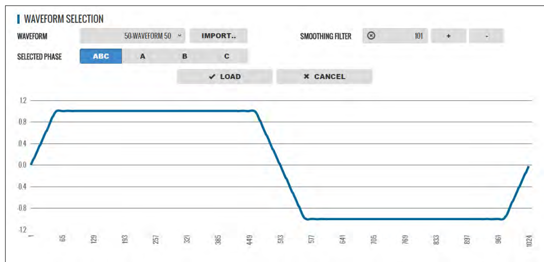
Figure 6-9: Same Waveform with maximum smoothing Filter Applied
