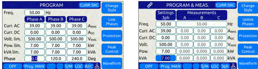
Figure 6-3: PROGRAM Screens Current Source Mode
