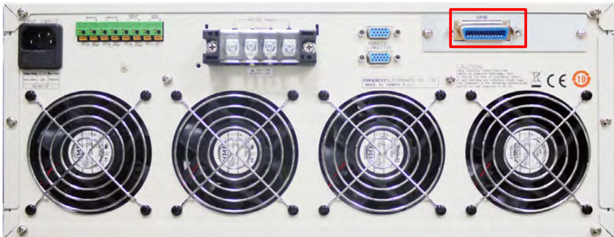
Figure 5-3: 3C Series Chassis Rear Panel – GPIB Option Location
