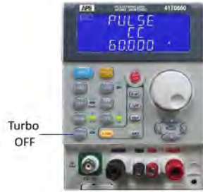
41T Turbo mode OFF Fuse Mode Test Result Screen
