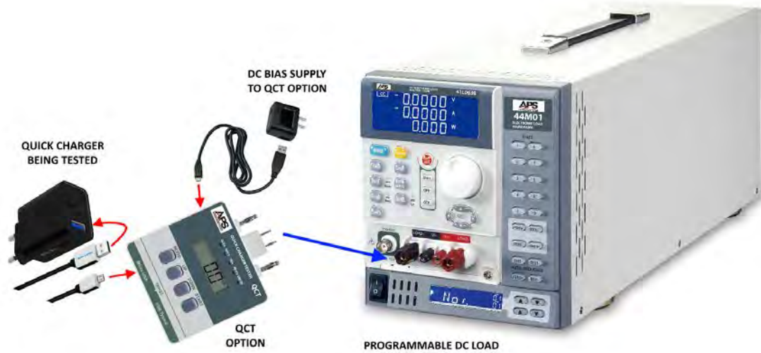
Figure 6-2: QCT Option and DC Load Test Setup
