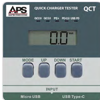
Figure 6-1: QCT Option Front Panel Display and Controls
