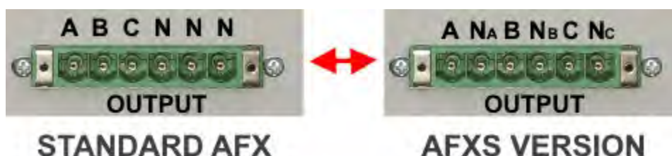
Figure 5-15: Standard ADF model vs ADF-W Model Output Connector pins
