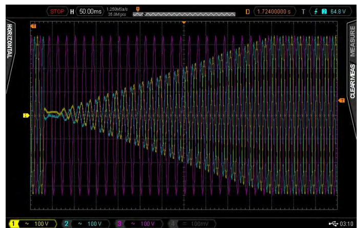
Figure 19: IEC 61000-4-34 Three Phase Voltage Variation Test
