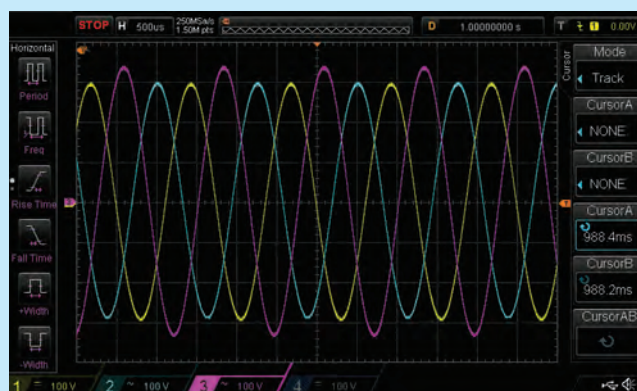
Three Phase Unbalance Voltage Test Captured
