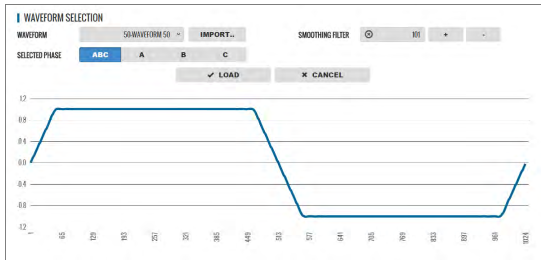
Figure 6-6: Same Waveform with maximum smoothing Filter Applied
