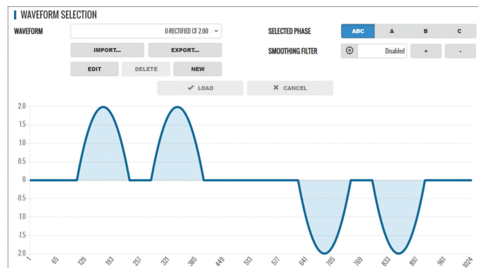
Figure 11: Three Phase AC Rectifier Current Waveform
